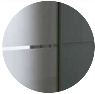
Sandblasted surface area with clear stripes
